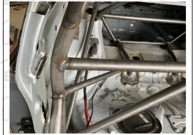
PHOTO 13 SHOULDER HARNESS ATTACHMENT - CO DRIVER
